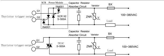
Note 1: According to the voltage and current of load, choose suitable varistor to protect the thyristor. A resistor-capacitor circuit (RC circuit) is needed for inductance load or phase-shift trigger output.
